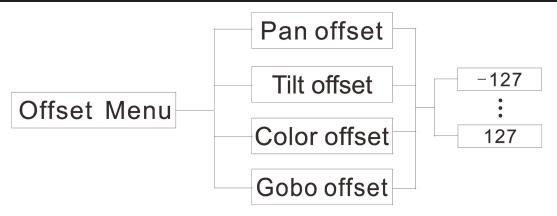
To enter the home position adjustment menu, press the ENTER button for at least 5 seconds. In this submenu you are able to adjust the original position of the pan position, tilt position, color wheel position, and gobo wheel position.
