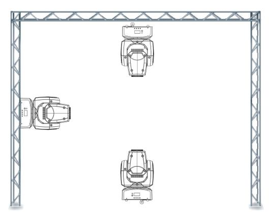
The Pocket Pro is fully operational in three different mounting posi-tions, hanging upside-down from a ceiling, mounted sideways on trussing, or set on a flat level surface. Be sure this fixture is kept at least 0.5m away from any flammable materials (decoration etc.). Always use and install the supplied safety cable as a safety measure to prevent accidental damage and/or injury in the event the clamp fails (see next page).
