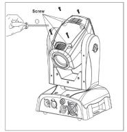
Unscrew the 4 screws located on the other side.
